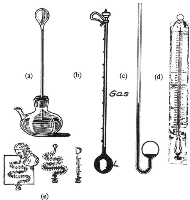
Figure 6 Thermometers in the seventeenth and eighteenth centuries: (a) Galileo's thermoscope; (b) the first sealed Florentine thermometer (1665); (c) Amonton's constant-volume thermometer (1702); (d) thermometer used by Celsius (1737); (e) the first clinical thermometers of Santorio (1612).
